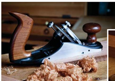
**New technology.** The "blade carrier" allows you to use the plane with or without a cap iron, and makes setting the cap iron a snap.
