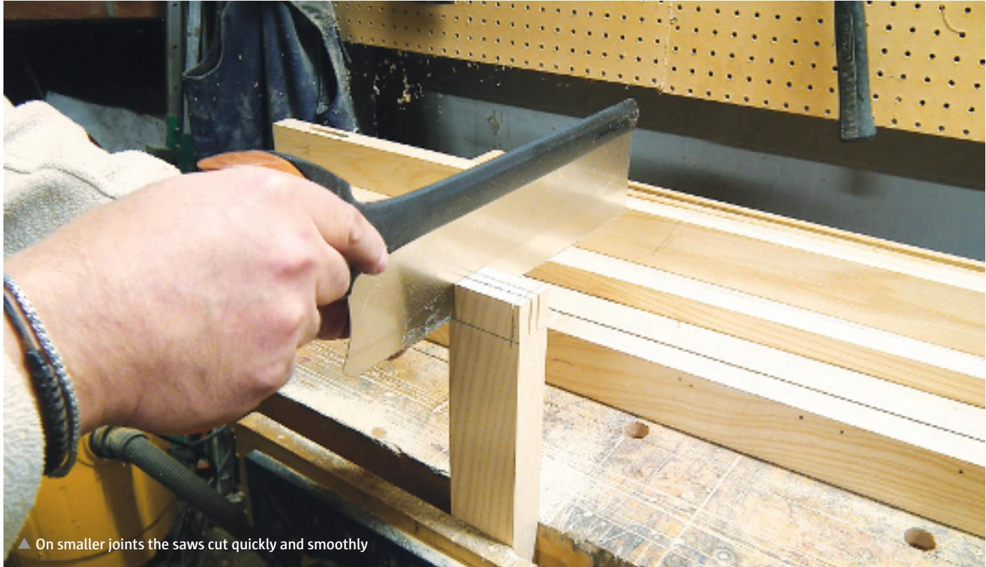
▲ On smaller joints the saws cut quickly and smoothly
