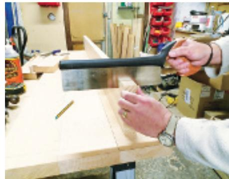
▲ Thick stock and deep cuts can take longer as the saws lack the weight of brass-backed models
