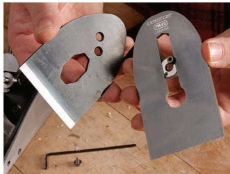
**Easy-to-set chipbreaker.** The chipbreaker registers on a round "blade carrier" attached to the blade, so you can quickly reattach the chipbreaker after sharpening the blade.
