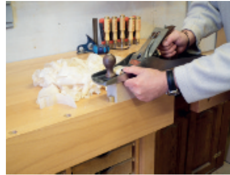
▲ When used with bench dogs, the vice can hold long lengths of timber on the worktop...
