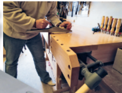
▲ ...or the jaws can be used conventionally to clamp workpieces solidly to the bench while you work them
