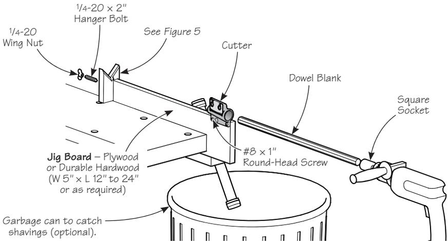
**Figure 3: Alternative dowel-making set-up.**
