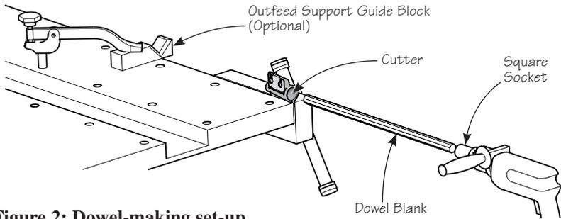
**Figure 2: Dowel-making set-up.**
