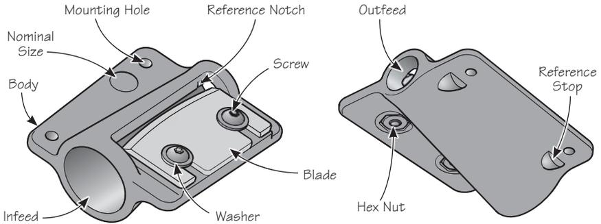
**Figure 1: Dowel and tenon cutter components.**
