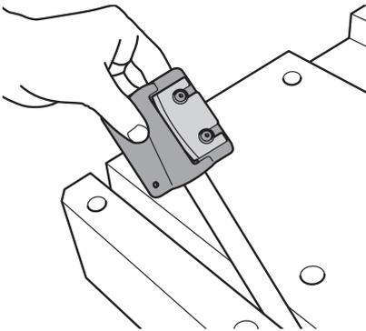
**Figure 9: Using a vise, turning the cutter.**
