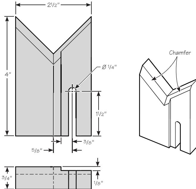
**Figure 5: Outfeed support V-block (adjustable).**
