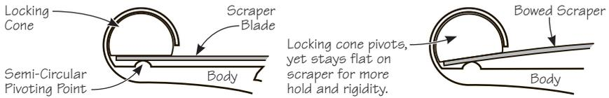
**Figure 2: Bowing the scraper blade.**
