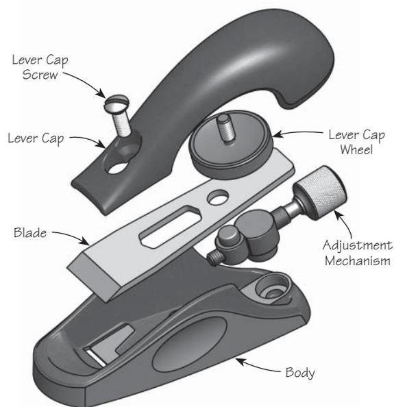
Figure 1: Pocket plane components.
