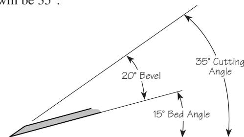
Figure 2: Blade geometry.
