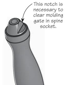
Figure 5: Notch detail.
