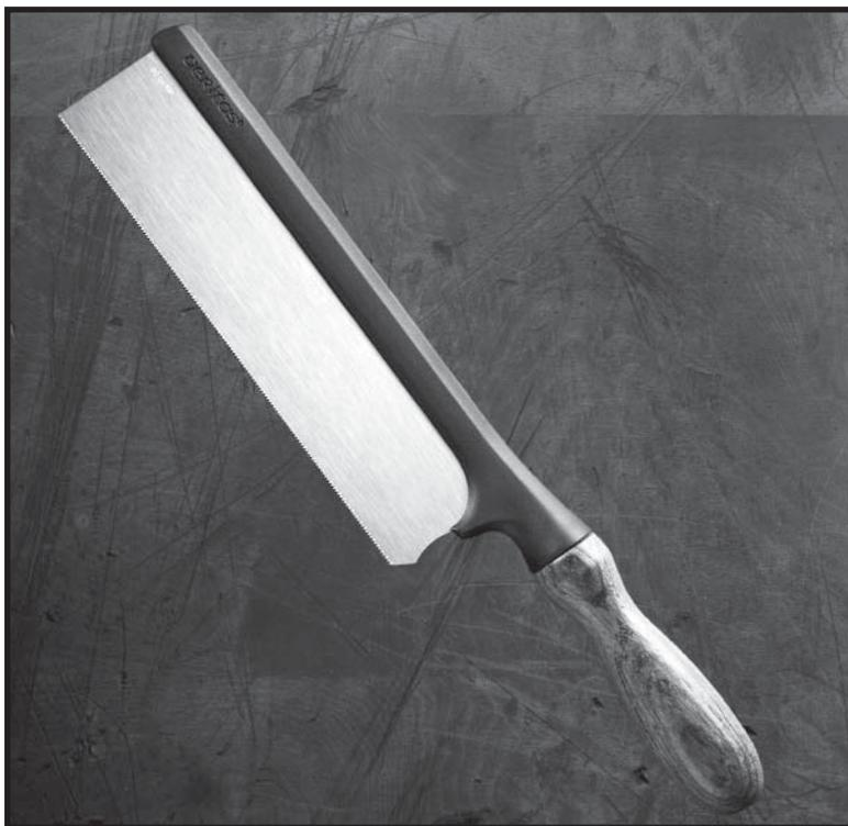
The Veritas® saws combine the best characteristics of the classic gent's saw with those of state-of-the-art materials and construction methods. The tooth pattern on the thin high-carbon steel blade provides a good balance between cutting action and surface finish. The stainless-steel/glass/polymer composite spine provides strength and rigidity.
