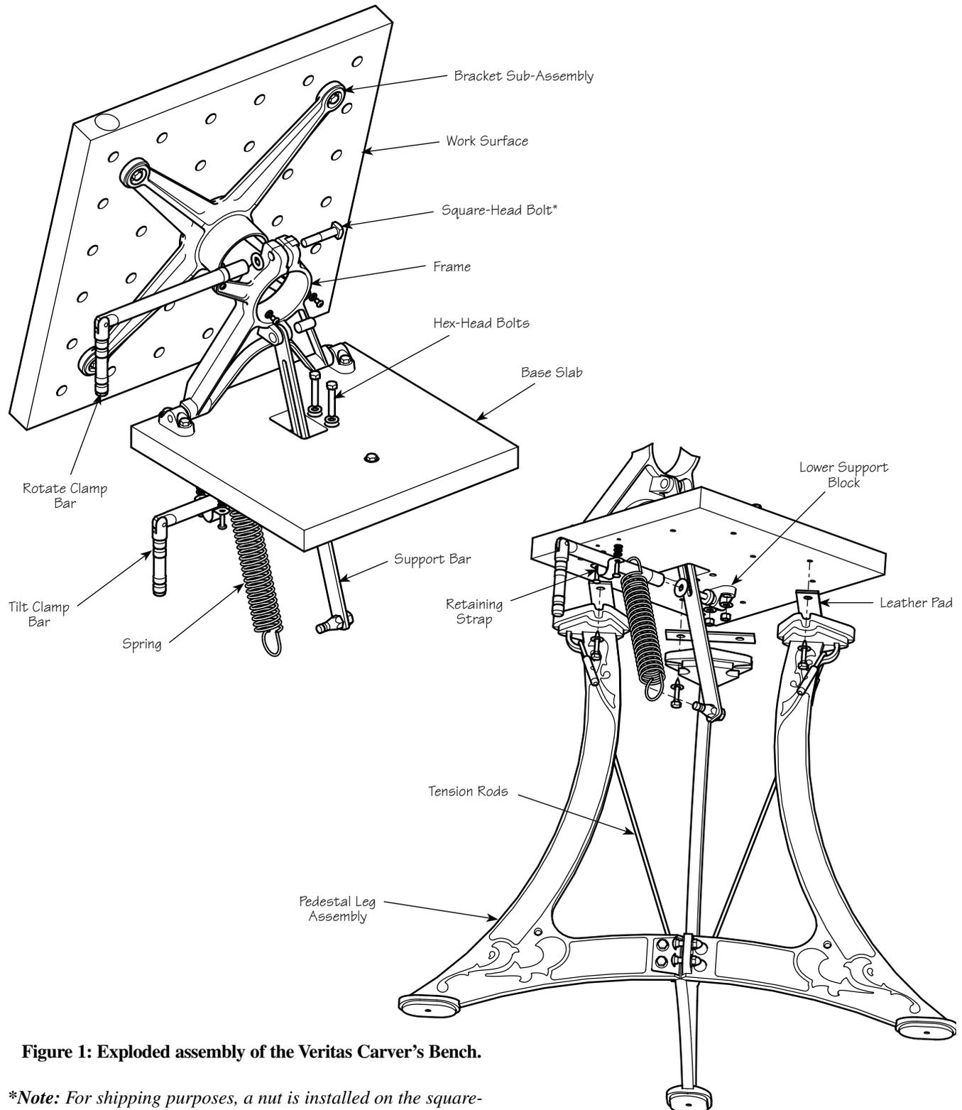
**Figure 1: Exploded assembly of the Veritas Carver's Bench.**
