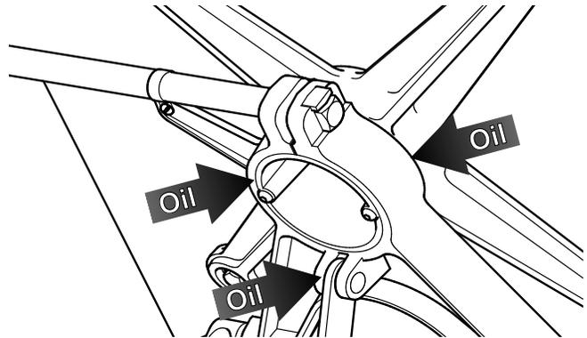
**Figure 16: Apply oil at these locations while rotating the work surface.**
