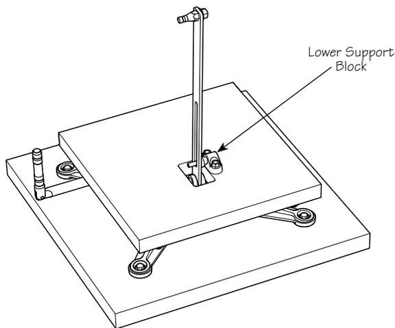
**Figure 7: Closed carver's bench top with lower support block installed.**
