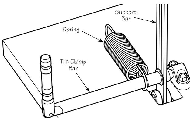
**Figure 9: Installing the spring. Leave the opposite end of the spring free.**
