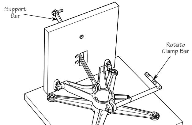
**Figure 4:** Carver's bench with support bar installed. Note orientation of support bar and rotate clamp bar.
