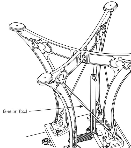
**Figure 12: Tension rod assembly.**
