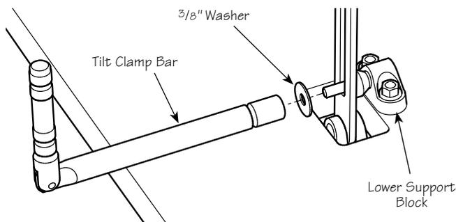
**Figure 8: Attaching the tilt clamp bar.**
