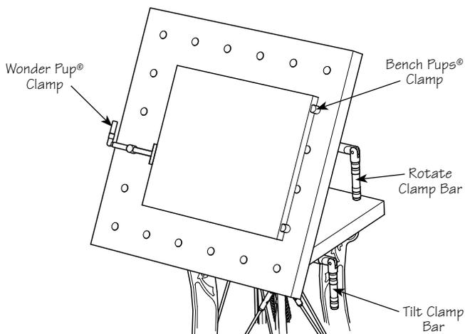
**Figure 15: Workpiece held in place with included Wonder Pup® and Bench Pups® clamps.**
