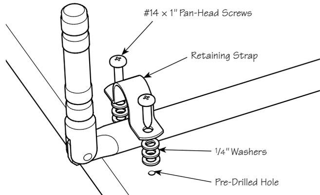
**Figure 10: Securing the tilt clamp bar retaining strap.**
