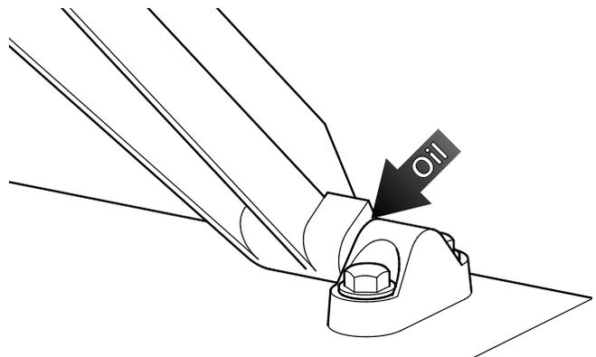
**Figure 17: Oil this location (both sides) while working the tilt joint.**
