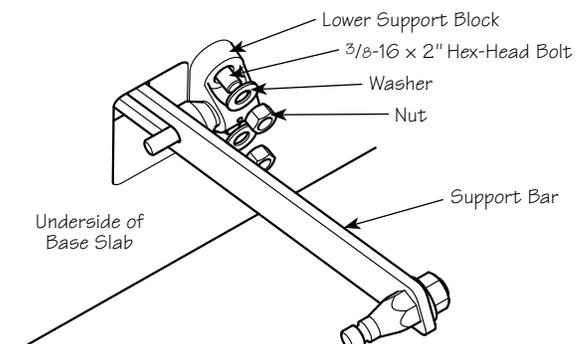
**Figure 6:** Lower support block assembly.
