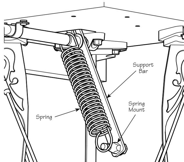
**Figure 14: Hook the spring over the support bar spring mount. Note: One leg has been removed for clarity.**
