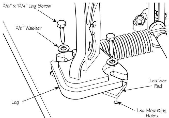
**Figure 11: Attaching pedestal legs to carver's bench top.**
