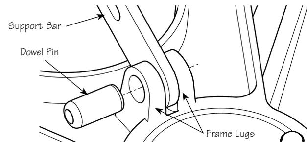
**Figure 5:** Attaching the support bar.
