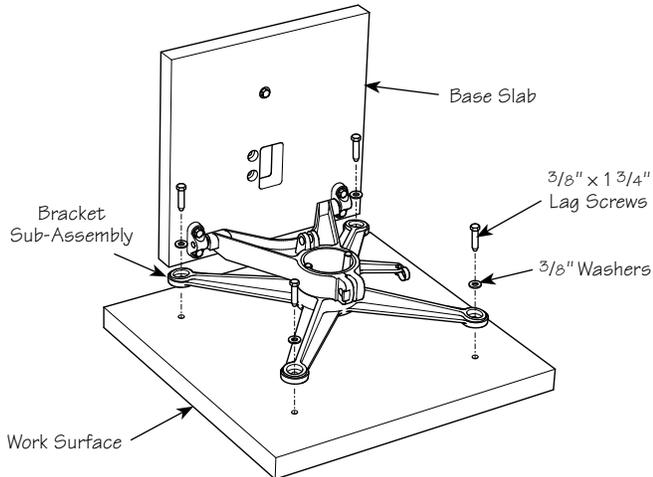
**Figure 2:** Securing the work surface to the bracket sub-assembly. Base slab lifted to show carver's bench frame.
