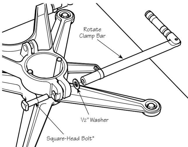
**Figure 3:** Installing the rotate clamp bar.
